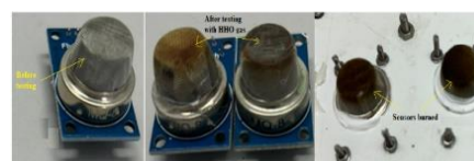
(a) Before testing, (b)-(c) After testing Fig. 9 (a) The Hydrogen Sensor before testing, and (b) and (c) the physical damage to the Hydrogen Sensor after exposure to high concentrations.
