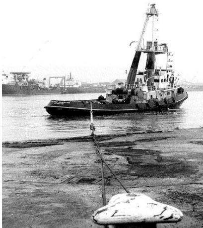
FIG 1 Bollard test arrangement
