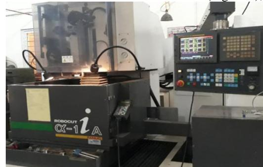
Fig. 1: Wire-cut electrical discharge machine
