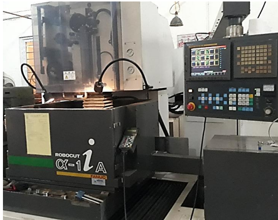
Fig. 1: Wire-Cut Electrical Discharge Machine
