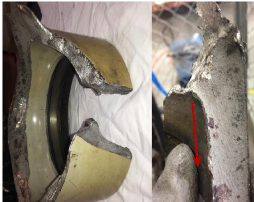
Fig 2: Fractured Hubs from the Inboard Wheel Half
