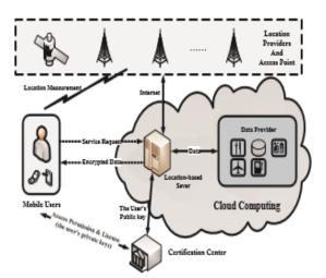
Figure 1: Location-based service architecture.
