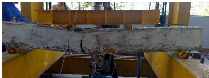
Fig 3.2 Cracking pattern for SFRC Beam
