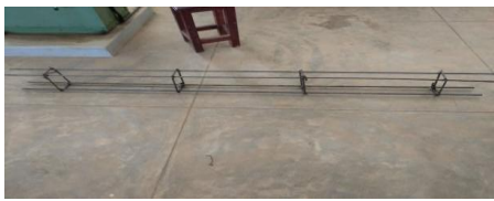
Fig 2.1 Reinforcement Details of FRC Beams
