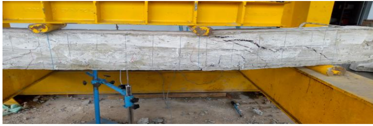
Fig 3.4 Cracking Pattern of GFRc Beam
