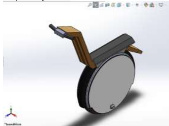
Fig. 2 Electric Unicycle's Design by Computer (Solidworks)
