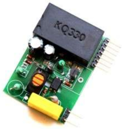
Figure 2: Power Line Carrier Communication Modem.
