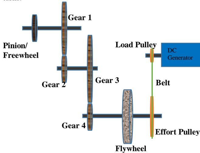
Figure 6. The gear system showing the arrangement of the pinion/freewheel, gears, flywheel, pulley belt, and the DC generator
