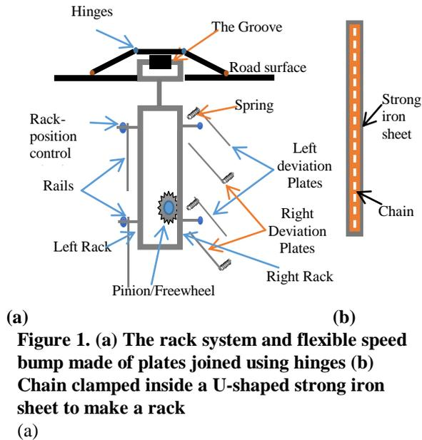
**Figure 1. (a) The rack system and flexible speed bump made of plates joined using hinges (b) Chain clamped inside a U-shaped strong iron sheet to make a rack**
