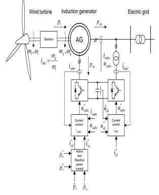
Fig.1. Wind turbine control system with DFIG
