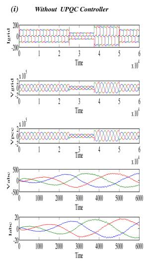
Fig.4 voltage and current waveform of load side, source side and point of comman coupling without controller
