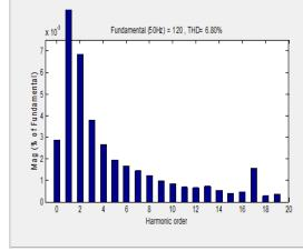
Fig.7 THD of Source Current with PI Controller
