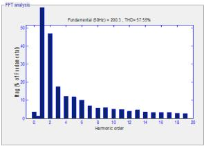
Fig.5 THD of Source Current without Controller
