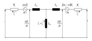
Fig.2 Equivalent diagram of the induction machine for dynamic states
