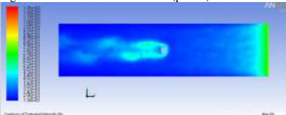
Fig 25. Contours of Turbulent Intensity (%)
