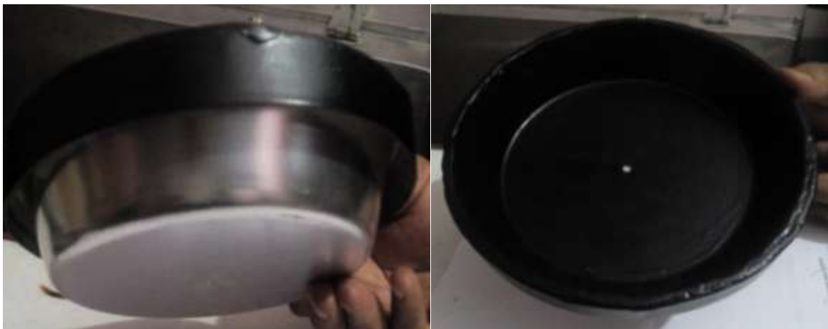
Fig. 3 A design of lid used in study - frustum of cone shaped lid
