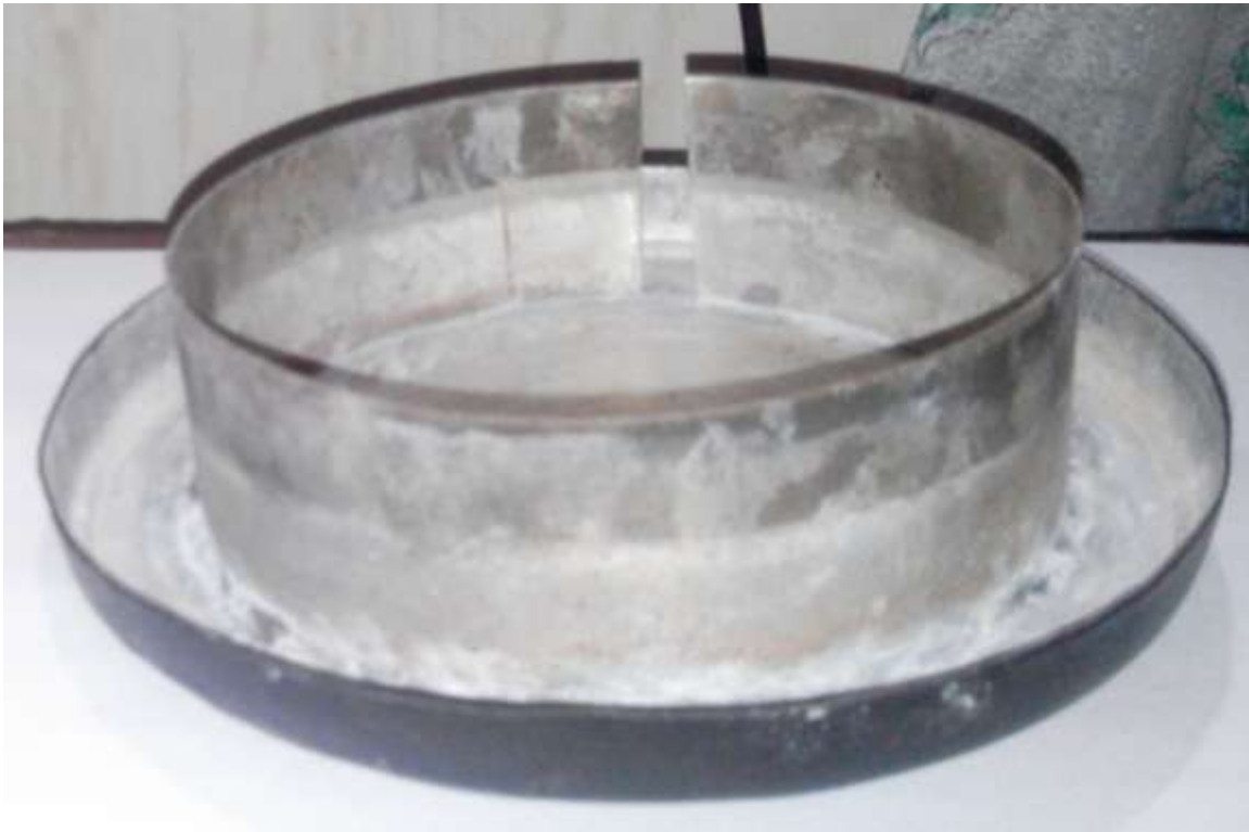
Fig. 2 Special design of lid used in the study in which a circular ring of aluminium strip welded to the inner side of lid of aluminium pot
