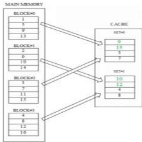
Fig. 2.2. Cache replacement within 4-way set-associative Cache
