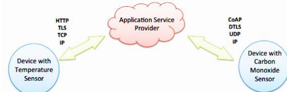
Figure 2. Device-to-cloud communication model diagram.
