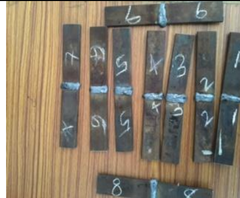
Fig 6: Work Pieces after Welding
