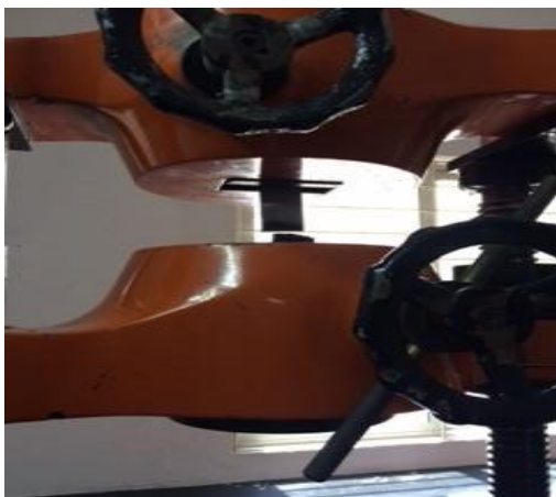
Fig 8: Joint breaking on UTM machine
