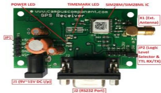
Figure 6: Pin description of GPS module.
