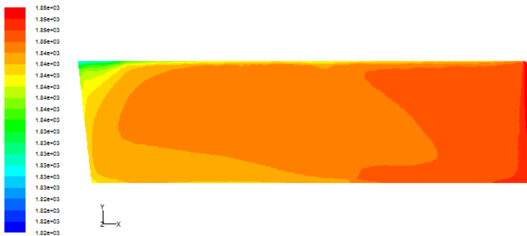
Fig. 7a Temperature distribution in the vertical plane through the inlet center
