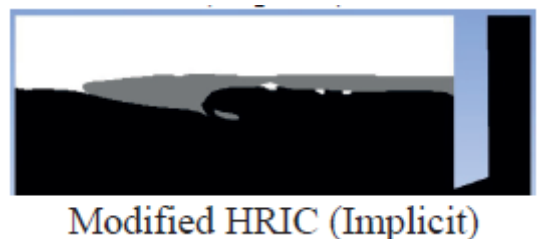
Fig. 6 Illustration of the slag entrapment[7] The view image in Fig. 6 is very similar to the results of the present simulation (Fig. 7c), in which the Modified HRIC (Implicit) procedure is used. [7] Has used different discretization schemes of the interface tracking and got similar result to the
