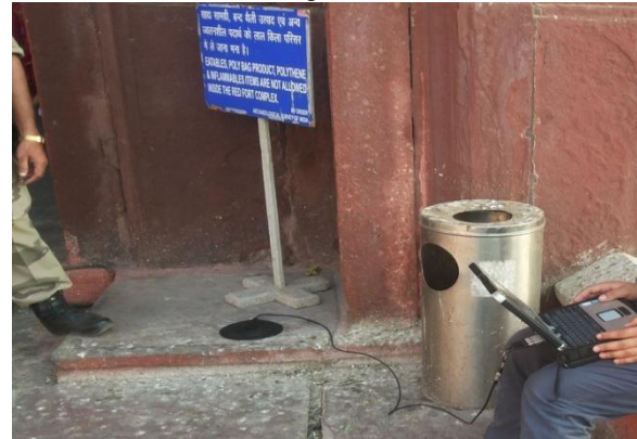
Figure 3: Triaxial accelerometer and sound book for Collection of data.
