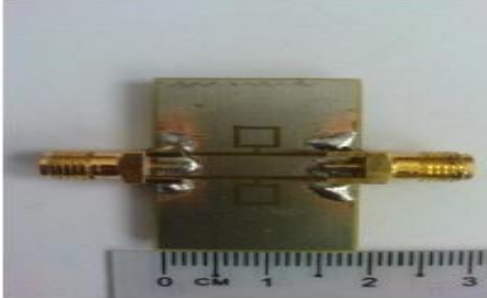
Figure 10: Reconfigurable CPW technology based resonator [13]
