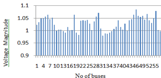
Graph 3.3 when fuzzy decision making technique is applying then graph of voltage is following
