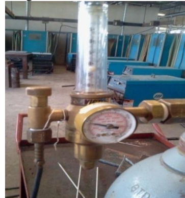
Figure 2: Single tube flow meter
