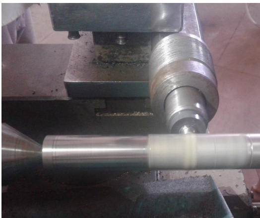
Fig 7 Ball burnishing operation for EN24 Steel
