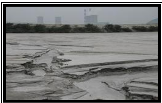
Fig.3.Wet disposal of Pond ash
