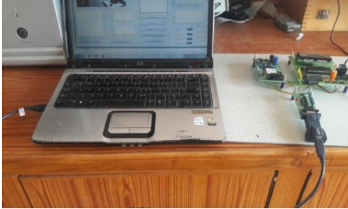
Fig 5.11: Interfacing of hardware setup with PC using RS232 Cable
