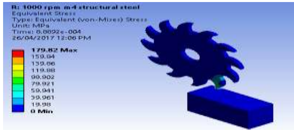
Figure 6: Stress results at 1000 rpm speed of M4 HSS and structural steel
