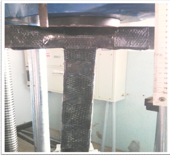
Fig 4.7 Experimental Analysis of I-Section Using CFRP Sheet
