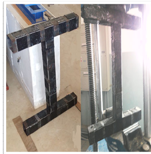
Fig 4.6 Experimental Analysis of I-section Using CFRP Sheet
