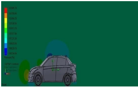
Fig 3.3.a: Pressure Contour with Vortex Generator
