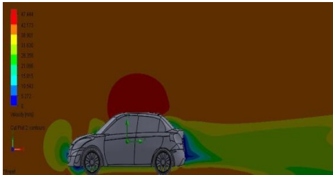
Fig 3.3.b: Velocity Contour with Vortex Generator
