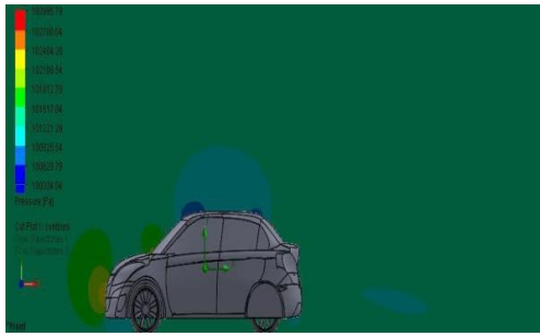
Fig 3.5.a: Pressure Contour with Tyre Cover
