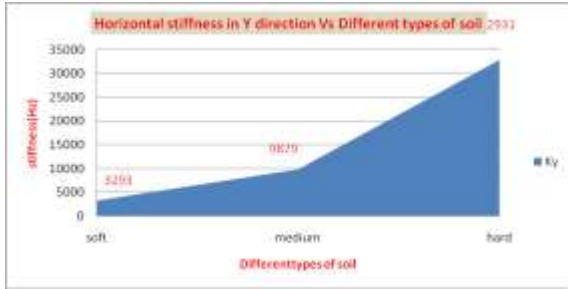
Chart 2 Horizontal stiffness in Y direction Vs Different types of soil
