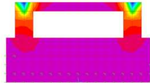
Figure 5 Maximum stress distribution in box foundation
