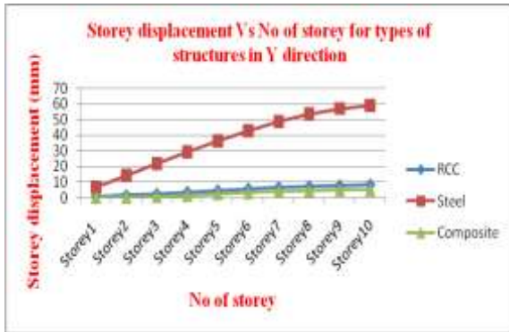
Chart 11:-Graph of storey displacement in Y direction for 10 storey building
