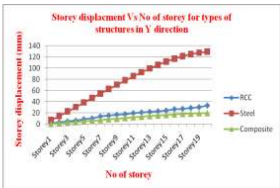
Chart 13:-Graph of storey displacement in Y direction for 20 storey building
