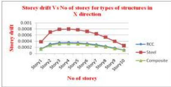
Chart 4:-Graph of storey drift of 10 storey building for EQx force
