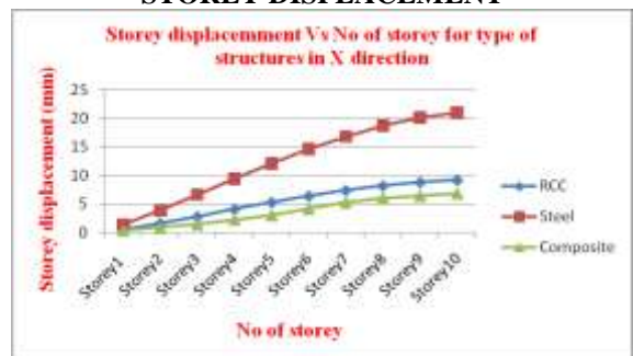
Chart 10:-Graph of storey displacement in X direction for 10 storey building
