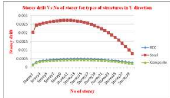
Chart 9:-Graph of storey drift of 30 storey building for EQy force
