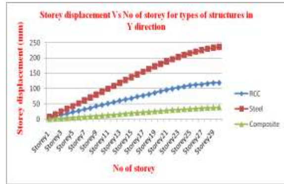
Chart 15:-Graph of storey displacement in Y direction for 30 storey building
