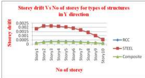
Chart 5:-Graph of storey drift of 10 storey building for EQy force
