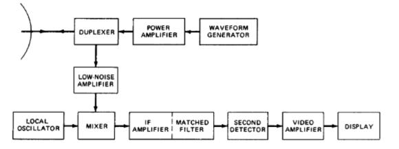
Fig. 2 Simple block diagram of radar
