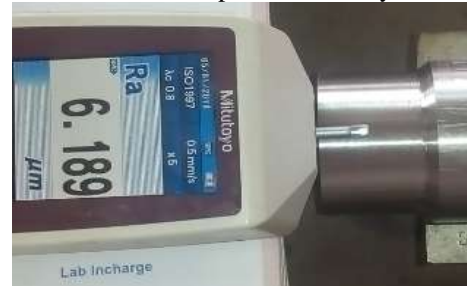
Fig 5: Stylus Movement on Work piece Material
