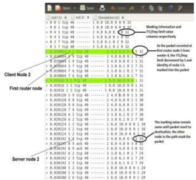
Fig. 5: Analysis of trace file of wired network simulation
