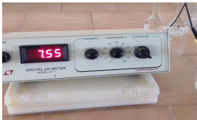
pH value is recorded for the entire sample using the pH meter
