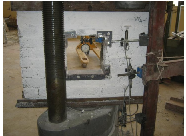
Figure (15): The used LVDT for measuring vertical deformation.
