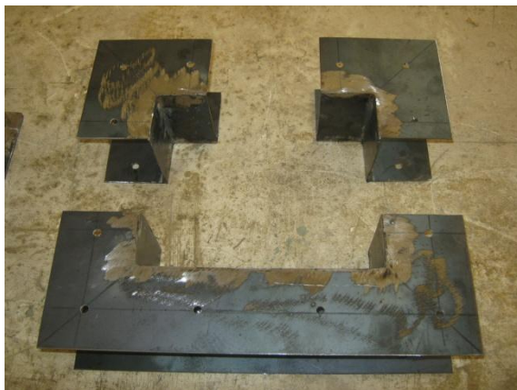
Figure (7): The used L&U-shaped steel plate.
