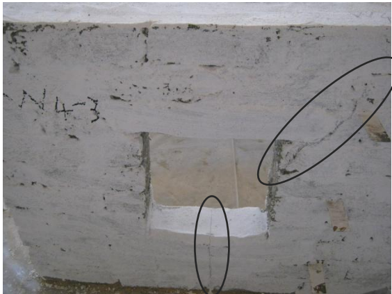
Figure (5): The crack pattern for tested wall specimen before rehabilitation
