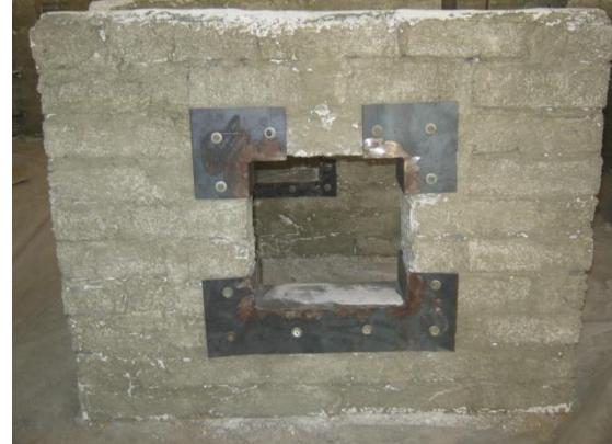
Figure (11): Details of the used rehabilitation technique using (2x80mm) L&U-shaped steel plate inside opening corners welded with U & L-shaped steel plate.
