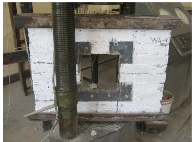
Figure (16): A steel beam as C-channel for transfer the load to wall.
