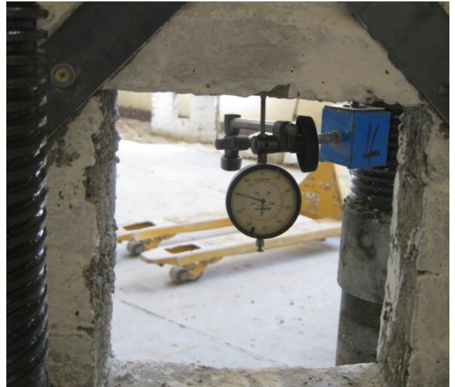
Figure (14): The used dial gauge for measuring lintel deflection.
