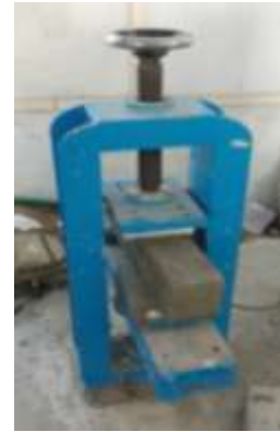
Figure4 Flexural Strength Test
