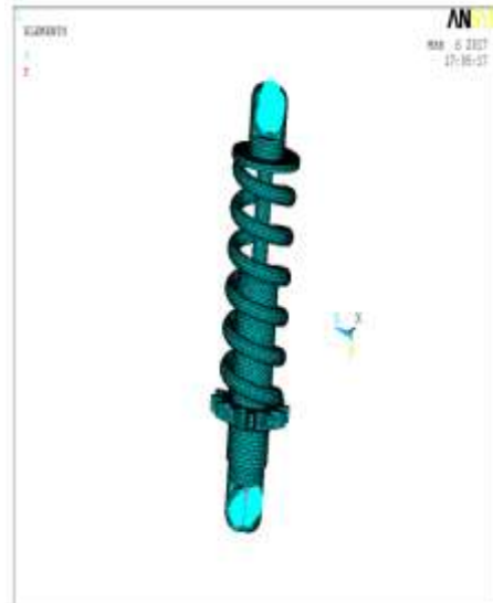
Fig.11. Static Load applied on tetra meshed model
