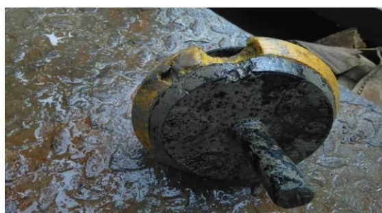
Fig 6. Damaged liner piston
