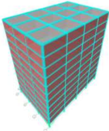
Figure 8 Model 4: G+10 RC first soft storey building with slab element 3D view
