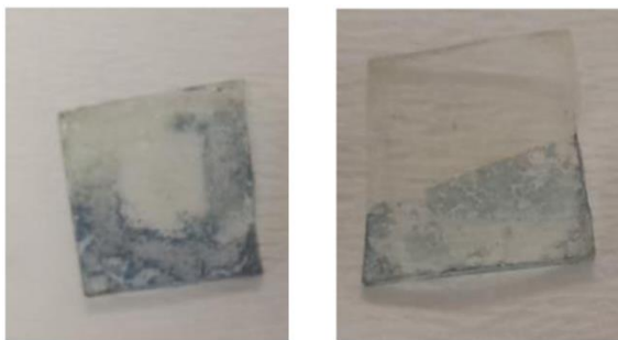
Figure. 4. Photographs of the Electrochromic WO 3 /ITO samples turned blue colour synthesized with Spin Coating at 3000 rpm and 6000 rpm respectively.
