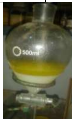
Figure 3 Biodiesel washing with hot distal water
