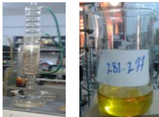
Figure 2 (a) Roselle seeds in Soxhlet (b) sample of Roselle oil extracted.
