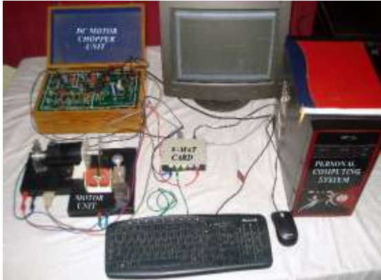
Fig. 1. DC motor speed control real time setup
