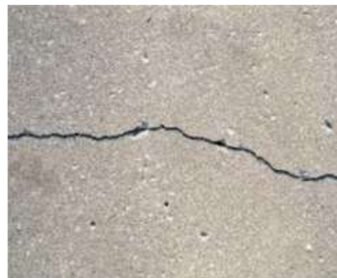
Fig. 13 Crack in Bacillus Licheniformis Sample after 28 days of Curing
