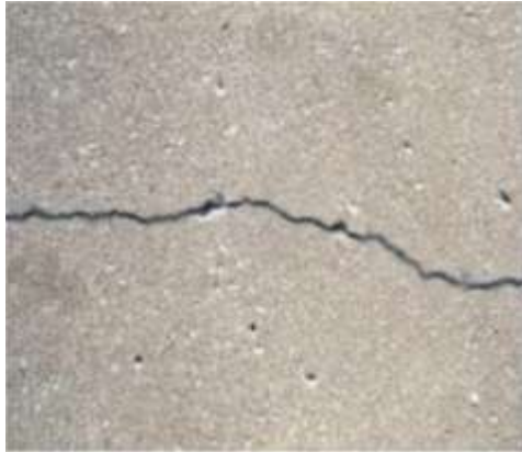
Fig. 14 Crack in Bacillus Licheniformis sample after allowing for Self-healing
