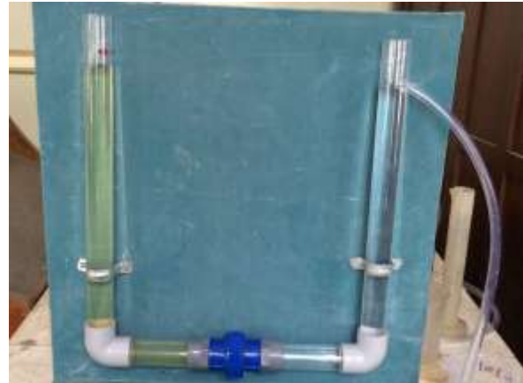
Fig 2: Experimental set up of Forward Osmosis
