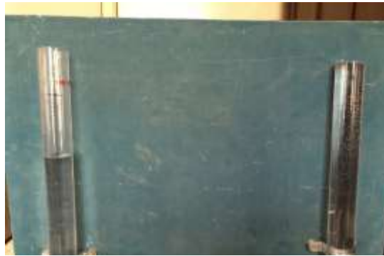
Fig 3: Changes in volume of Feed solution and draw solution after a period of 4 days
