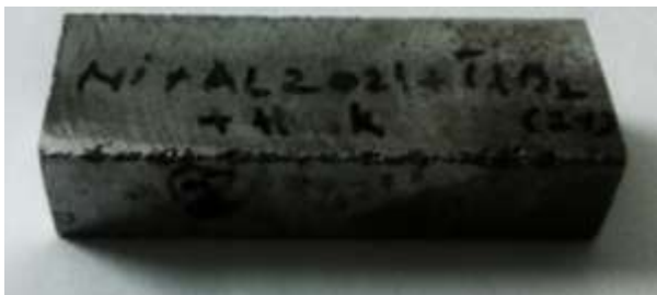
Fig 6 Raw material of Metal Matrix Composite: Al 2021 + TiB 2 + Ni + Husk material
