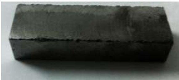
Fig 5 Raw material of Metal Matrix Composite: Al 6062 + TiB 2 + Ni material
