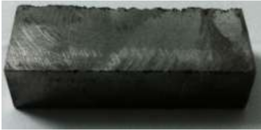
Fig 4 Raw material of Metal Matrix Composite: Al 6061 + TiB 2 + Ni + Fly ash material
