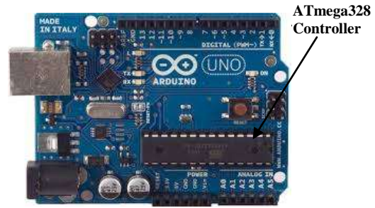
Fig.4: Arduino Uno board with ATmega328 Controller
