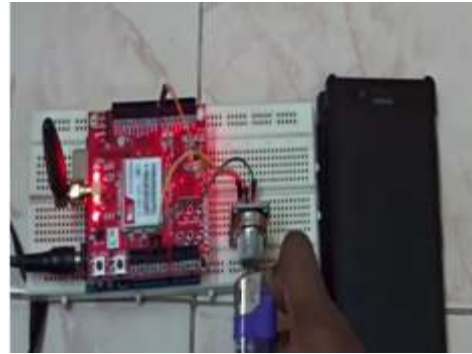
Fig.10a: Testing of the Gas leakage detection and alarming system
