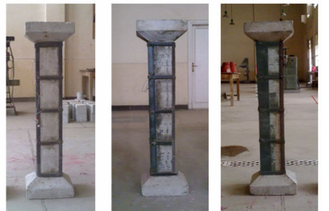
2 angles 20 \times 20 \times 2 mm in compression side and 2 angles 20 \times 20 \times 2 mm in tension side 2 angles 40 \times 40 \times 2 mm in compression side and 2 angles 20 \times 20 \times 2 mm in tension side 2 angles 60 \times 60 \times 2 mm in compression side and 2 angles 20 \times 20 \times 2 mm in tension side
