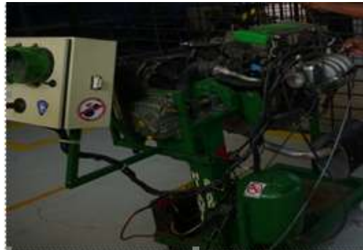
Fig. 10 Naturally aspirated engine- SP4H Proton connected to Engine Analyzer via the probes.
