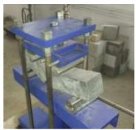
Fig-6: Flextural Test.
